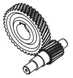
$$P_1 = \frac{M_2 \cdot n_2}{\eta \cdot 9550} \text{ [ kW ]}, M_2 \text{ [ Nm ]}, n_2 \text{ [ min}^{-1} \text{ ]}$$
